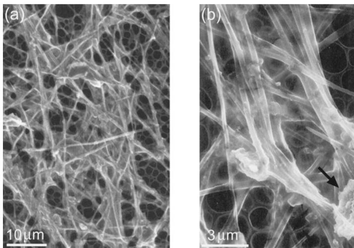
**Figure 1.1** (a) Scanning electron microscopy (SEM) image of the  $C_{60}$  NWs formed in a PZT sol containing  $C_{60}$ . The arrowed part of (b) shows a piece of PZT gel.<sup>4</sup>
