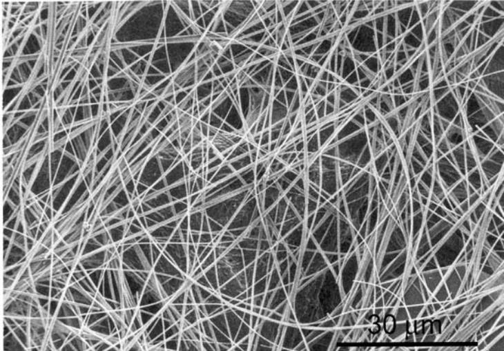
**Figure 1.2** SEM image of the C<sub>60</sub>NWs synthesized by the liquid–liquid interfacial precipitation method.
